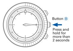
The manual reception can be performed whenever necessary irrespective of whether the automatic reception function is turned on or off.
