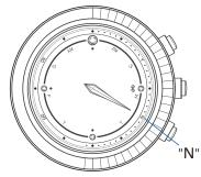
Press and hold Button A for more than 2 seconds. The hour and minute hand point to "Y" or "N" to indicate the result of the last reception performed in the past 24 hours for 5 seconds.
