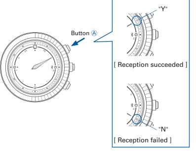
% If no reception succeeded or no communication was performed in the past 24 hours, the hour hand and minute hand point to "N."
