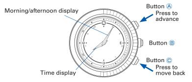
(3) Once you have finished setting the part dual time, press Button (B). The minute hand shows the "minutes," and then after 10 seconds, the display returns to show the time.
